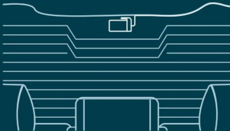
**7** Attach the camera to the rear window in a place where the view is not obstructed. Place the rear camera in such a way that the adhesive edge is on the right side as shown in the image above.
